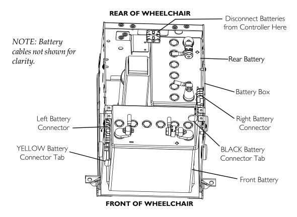
FIGURE 10.4 Installing Batteries
